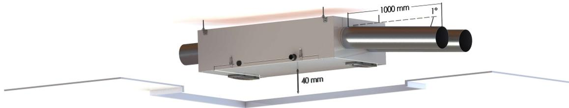
*Figure 4. Air intake duct connection diagram*
