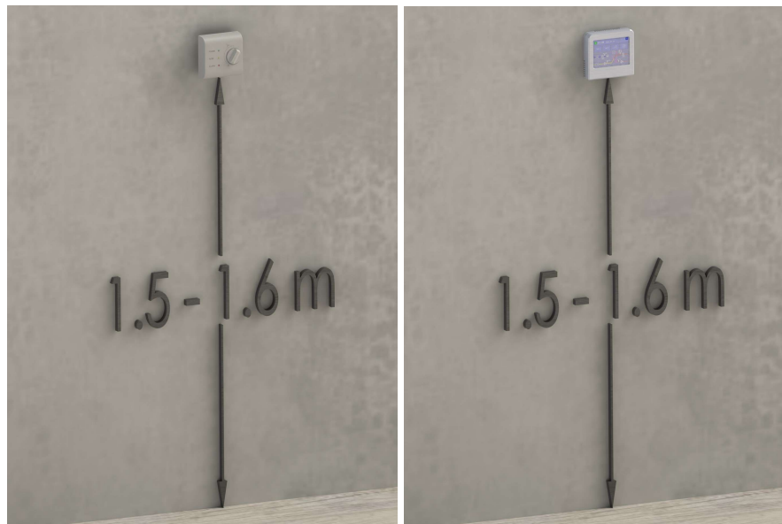
Figure 7. Installation of the control panel
