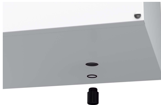
Figure 4. Installing the condensate drain
